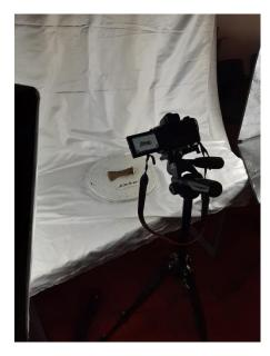
We had quite the nice setup for that, using once again a turntable and also the non-reflective coating spray that was presented to us before. I was very excited to be able to finally use it. I also had learned a lot about the workflow and since we were shown the specifics steps needed to merge two sides of an object so the model is whole, I could apply that knowledge to the working process whilst I was taking pictures.
