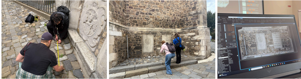
Photogrammetry data capture at Petrov and processing in RealityScan.
